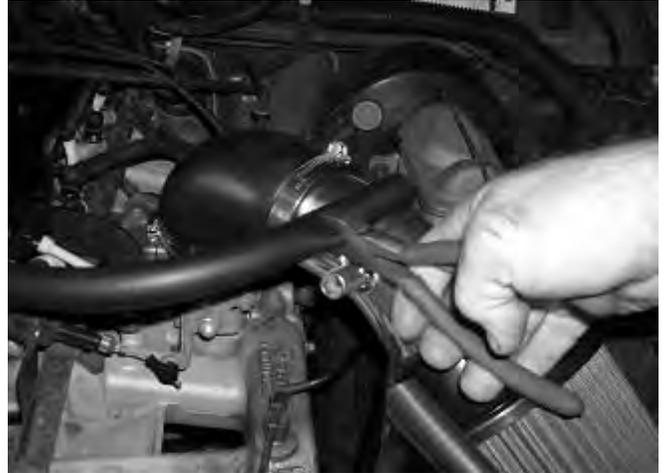
7. Secure the small vacuum line with a zip tie as shown. Attach the breather hose to the charcoal canister.
