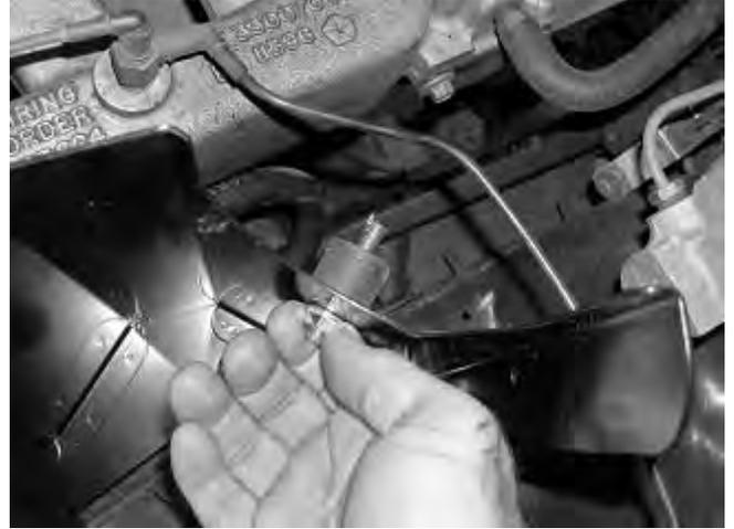
4. Install small edge trim around the intake tube area. Install the intake tube, securing with a hose clamp.
